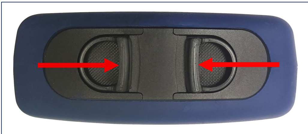
Figure 7 Squeeze latches together to release the battery cover
