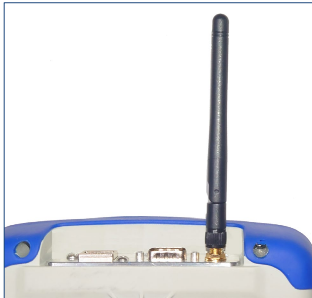
Figure 17 LR Bluetooth® antenna (left) and attached to the Washington (right)
