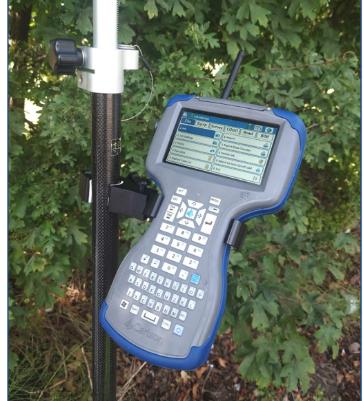
Figure 16 Pole mount and the Washington clamp (left) and mounted on a survey pole (right)
