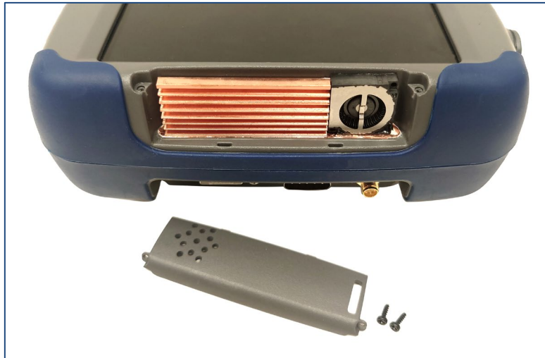
Figure 10 The Washington with the fan cover removed
