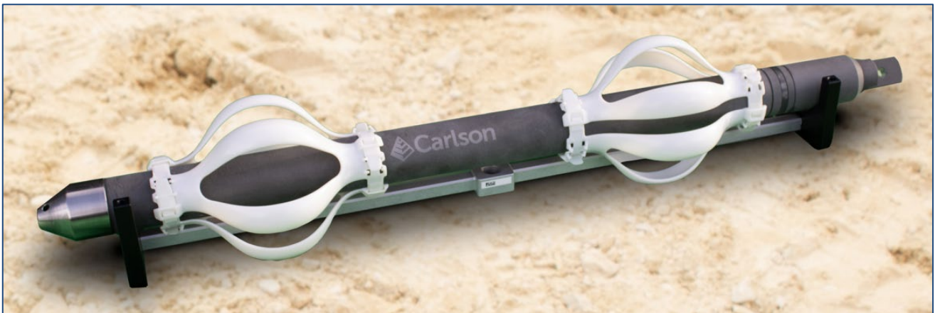
Figure 10 Boretrak360 probe fitted with centralisers for uphole deployment
