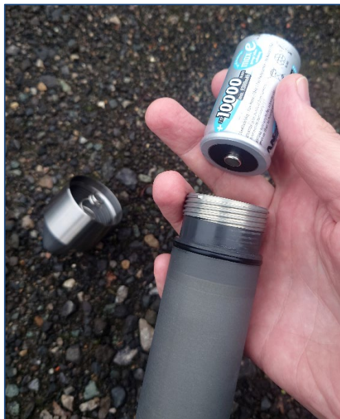
Figure 2 Positive battery terminal faces inward
