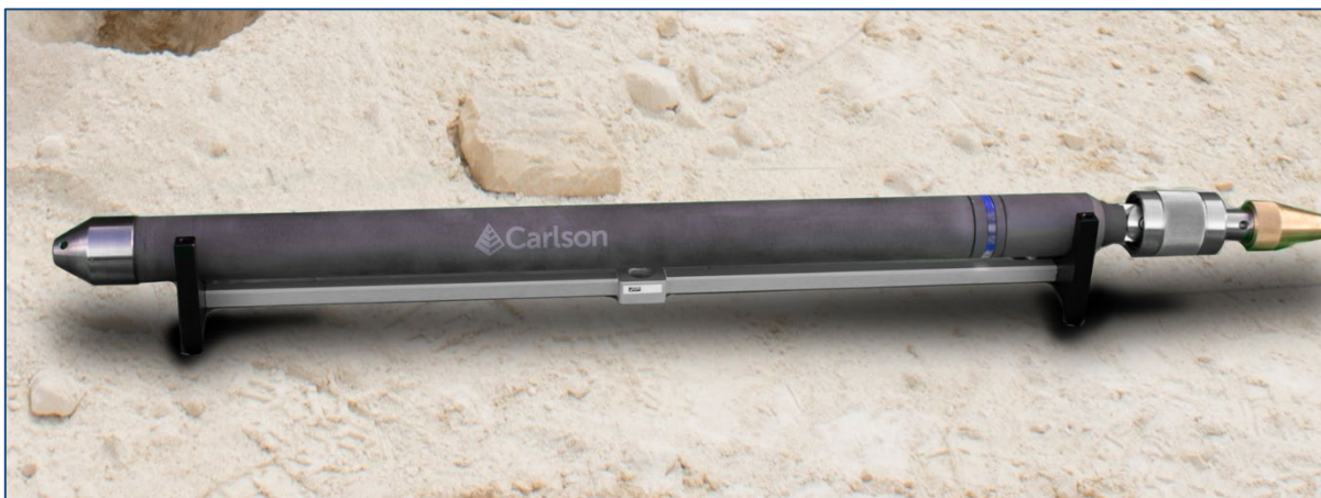
Figure 7 The Boretrak360 probe on the alignment jig
