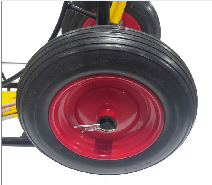
Figure 18 Securing the wheels with a cotter pin
