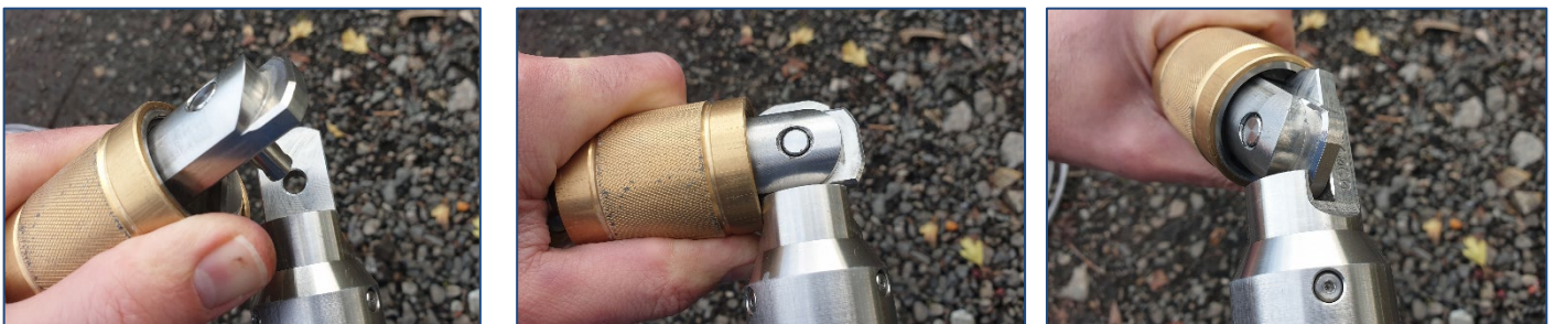
Figure 28 Connecting the deployment adaptor to the probe
