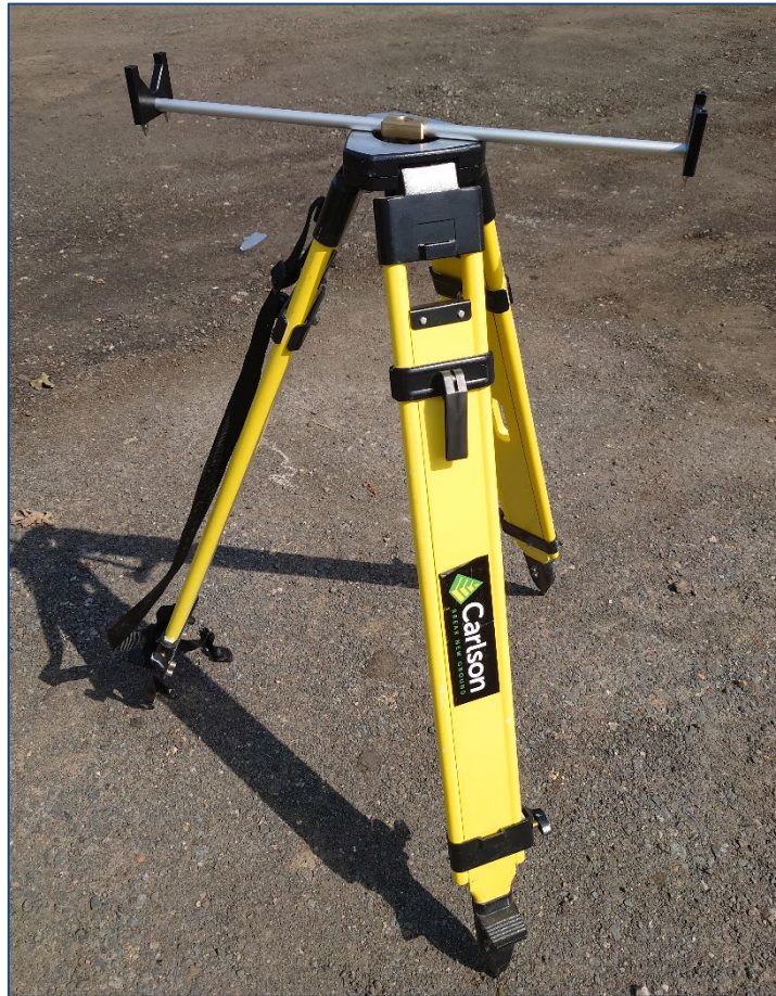
Figure 8 Gyro alignment jig mounted on a survey tripod
