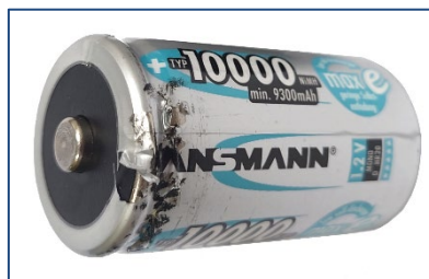
Figure 3 An example of a battery with a damaged outer coating. This battery should not be used in the Boretrak360 probe
