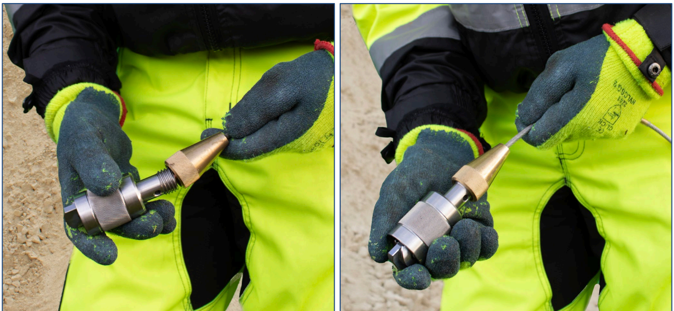
Figure 25 Screw the deployment adaptor firmly onto the deployment device
