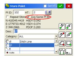
The screen shown below appears if GNSS Analysis is on, Store GPS vectors is on and Store GPS Accuracy in Raw File in on. So the Store Points screen itself shows, in effect, the same dialogs as appear in Point Average, whenever "Avg Same Pt ID" is on.
