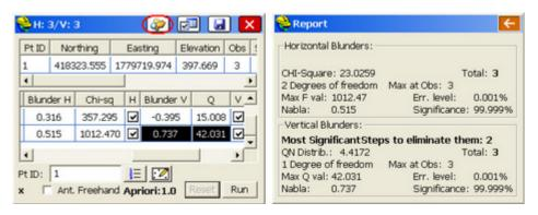
Start by entering the Point ID in the lower left of the dialog to study. Press Enter after selecting the point for the data to appear. The "worst" blunder is identified by highlighting to the left of the H or V column. So in this case, click of the V to the right of the highlight. Prior to doing so, if you click the Report icon (highlighted with red circle), you see the Report at right which shows the high F Value for the horizontal component and also high Q value for the vertical component.
