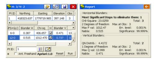
Notice how the Q value came down after removing the first vertical reading.
