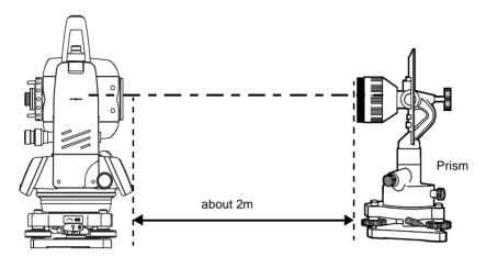
2) Sight through the eyepiece and focus to the prism. Then center the prism on the cross hairs.
