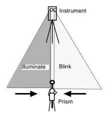
Once you have determined that both of the LED's are equally bright, you are on-line with the instrument.
