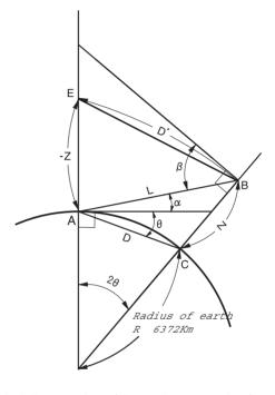
The conversion formula for horizontal and vertical distances is as follows when correction for refraction and earth curvature is not applied.
