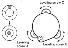
2 Turn the leveling screw C to bring the bubble to the center of the circular level.
