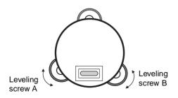
2 Rotate the instrument 90° (100g) around its vertical axis and turn the remaining leveling screw or C to center the bubble once more.
