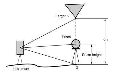
1) With prism height (h) input (Example :h=1.5m)
