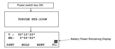
• Confirm the battery power remaining display. Replace with charged battery or charge when battery level is low or indicates "Battery empty". see Section 2.4 "Battery Power Remaining Display".
