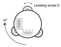
3 Repeat the procedures 1 and 2 for each 90° (100g) rotation of the instrument and check whether the bubble is correctly centered for all four points.
