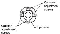
3)Shift the vertical cross-hair line and coincide it with Point D, by revolving the left and right capstan adjustment screws with the adjusting pin.Upon Capstan completing the adjustment, repeat the checking adjustment operation once more.
