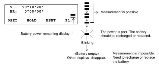
Note: 1 The battery operating time will vary depending on the environmental conditions such as ambient temperature, charging time, the number of times of charging and discharging etc. It is recommended for safety to charge the battery beforehand or to prepare spare full charged batteries.
