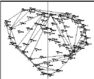
Select Lines, PLines, and/or 3DFaces that define the surface. Select objects: Pick the perimeter polyline and newly create triangulation lines
