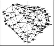
Select the points and barrier lines to Triangulate.
