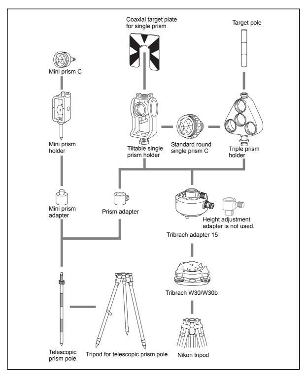
Figure 8.2 Prism reflector side
