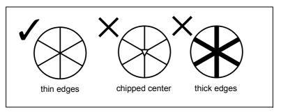
As the Nivo series is extremely sensitive, multiple reflections on the prism surface can sometimes cause a significant loss in accuracy.
