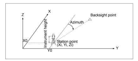
To enter the azimuth angle to the backsight point, press 2 or select Angle in the Backsight screen.
