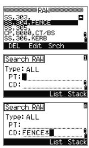
To search by point type, move to the Type field and use < or > to change the selected point type. The options are ALL, ST, SS, SO, CP, CO, CO(SY), and CO(RDM).
