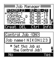
When you enter a point name or number, the system searches in the current job first. If the point is not found in the current job, the search is automatically extended to the control job. If the point is found in the control job, the selected point is copied to the current job as a UP record.
