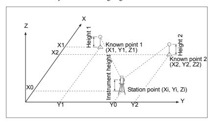
You can use a maximum of 10 points in a resection. Measurements can be distance and angle, or angle only. Calculation starts automatically when enough measurements are taken.
