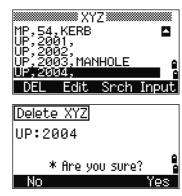
You can also delete coordinate data by pressing the DEL softkey in the detailed display screen for the record.
