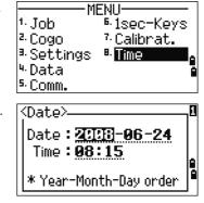
If the highlighted part of the field (for example, the year) is already correct, you can just press [ENT] to use the current value. For example, if the date is already set to June 24, 2008, and you want to change the date to June 18, 2008, press ENT ENT 1 8 ENT.
