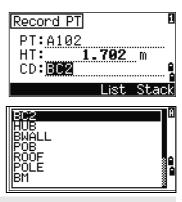
When the instrument is rebooted, the code stack is cleared.
