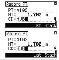
When the cursor is in a height (HT) field, only numeric input mode is available. Pressing MODE has no effect when the cursor is in a HT field.
