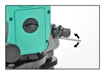
Repeat from Step 2. For laser plummet adjustment, a cap needs to be removed.
