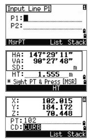
When you move the cursor to a field, the current or default value appears in inverted text (this is the default "Replace All" input mode).
