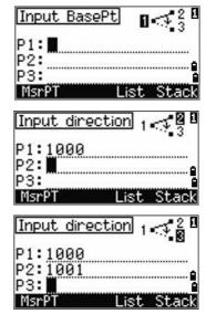
When you press the MSR softkey, a temporary measuring screen appears. Sight the target and press [MSR1] or [MSR2] to take a measurement.
