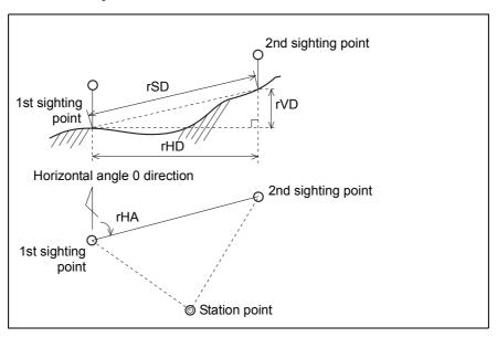
rSD Slope distance between two points rHD Horizontal distance between two points rVD Vertical distance between two points rV% Percentage of grade (rVD/rHD) × 100% rGD Vertical grade (rHD/rVD):1 rAZ Azimuth from first point to second point
