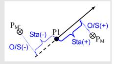
To calculate the coordinates of the point (PM), press [ENT] in the dVD field. You can change the Z coordinate here.
