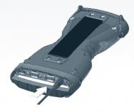
Plug battery charger into wall outlet, then into the unit.
