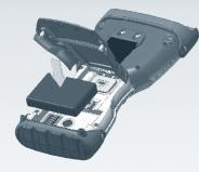
Insert the battery pack(s) so battery contacts match up.
