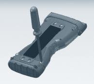
Use edge of a key or screwdriver to open battery compartment.\*
