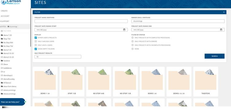
Set up a project in Carlson Photo Capture by naming it, choosing the desired output unit of measure and the correct output coordinate system projection.
