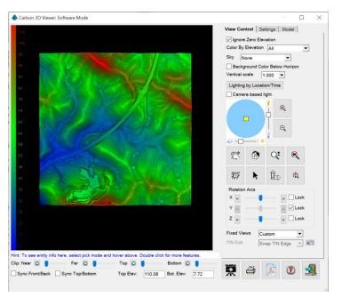
One example of using this data would be to draw contours for adjoining information or to obtain an approximate "lay of the land" (as this data has not, in most cases, been verified by a survey on the ground).
