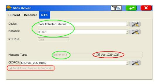
By <u>checking ON</u> the "Use 1021-1027" command, the user can activate the RTCM decoder in SurvCE. The messages coming from the caster will be analyzed from the very first connection to the mount-point. If the mount point is providing 1021, 1023 or 1025 messages, SurvCE will prompt the user, within the next few seconds after linked to the caster using Rover Setup, with the "RTCM messages Alert" dialog explained in the next chapter.
