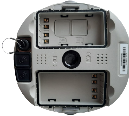
Figure 2-3: Battery compartment door removed
