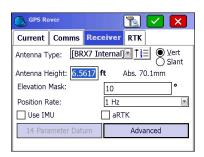
12) Tap the RTK tab and set it for "Device: **Internal Radio**" and make sure to check the box next to "Use any Base ID"
