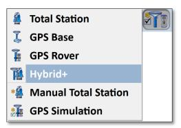
If you have not purchased the Hybrid+ module, you will be prompted to temporarily enter demo mode with the Hybrid+ module to try. Demo Mode will only allow a maximum of 15 points. You can revert to your full registered copy of the software by exiting and relaunching the software.
