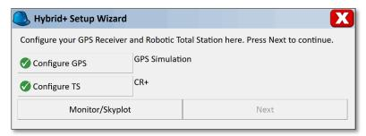
Next, the wizard will guide you through setting your GPS and RTS heights. Measure the height of the prism (from the tip of the pole to the center of the prism) and measure the height of the GPS receiver (from the found to the reference mark on the antenna, slant or vertical). Enter in these values in the screen.
