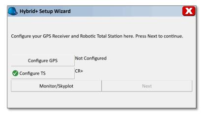
Configure the GPS as you normally would, ensuring a valid RTK correction link. Once the GPS receiver is configured, both buttons will show green check icons. Press 'Next' to continue.
