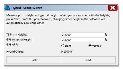
The software will now calculate the fixed offset between the center of the prism and the GPS receiver. From this point forward, changing either height (GPS or RTS) will automatically adjust the other using this fixed offset value. Press 'Next' to continue.
