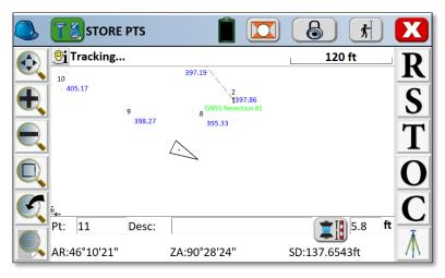
Within the Store Points screen, each time a point is stored with the robotic total station, the GPS measurement is collected at the same time. A localization will be formed in the background by analyzing all measurements pairs and selecting the best quality measurements.
