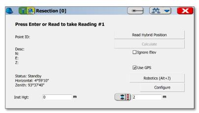
When you are satisfied with your resection, press 'Calculate' to view your results and store the calculated position of the robotic total station. The software will then set the orientation angle on the robotic total station and return to the wizard. The next step is to 'Perform a Cross-Check'. Cross-check will measure a position simultaneously using the robotic total station and GPS receiver. It will then compare the coordinates match based on the displayed tolerances.
