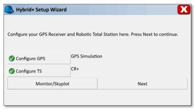
Next, the wizard will guide you through setting your GPS and RTS heights. Measure the height of the prism (from the tip of the pole to the center of the prism) and measure the height of the GPS receiver (from the ground to the reference mark on the antenna, slant or vertical). Enter in these values in the screen.
