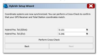
Cross-check tolerances can be augmented within this screen. Perform a Cross-check by pressing 'Perform Cross-Check'. Once setup is complete, the software will use these tolerances to detect any unacceptable deviations between the RTS and GPS positions. If an unacceptable deviation is present, a warning screen will pop-up to warn the field engineer.
