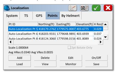
Press the green check to finalize the auto localization routine. With the localization complete, the next step is to perform a Cross-Check. The software will direct the user to the cross-check procedure automatically.
