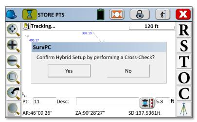
Click 'Yes' to perform a cross check. The Cross-check procedure will measure a position simultaneously using the robotic total station and GPS receiver and verify that the coordinates match. If the coordinates match within tolerances, the localization is good and the robotic total station and GPS receiver are on a matching coordinate system. Hybrid+ setup is complete.
