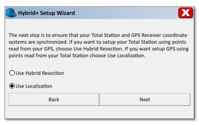
There are two methods of performing the localization for Hybrid+, localize manually and auto-localize. Localize Manually will proceed to the SurvCE localization screen where a localization may be created by measuring individual points and adding them to the localization. Auto-Localize will proceed to the Store Points screen and switch the active instrument to the robotic total station. The auto-localization will complete once enough points are measured.
