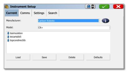
Press the green check to connect and return to the wizard. Both buttons should now have a green check to indicate the instruments are configured. Press 'Next' to continue.
