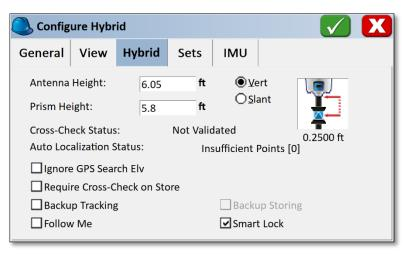
The screen shot above reflects the status of an Auto Localization routine before any points are stored. When enough points are stored the Auto Localization status will switch from 'Insufficient Points [0]'.
