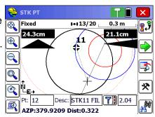
Note that the sensor icon in the top bar is now green, though the e-level is showing out of level.
