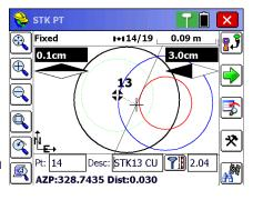
In this last image the e-level is off center, which indicates that the pole is tilted, but the green icon at the top lets the user know that the incline will be accounted for in the software.
