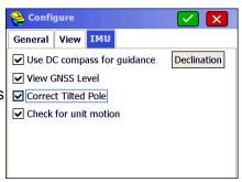
• <u>Use DC compass for guidance</u> – this setting improves navigation directions by using the internal compass of data collectors if possible. It may be necessary to calibrate the internal compass of your data collector. The Magnetic Declination button allows you to confirm the calculated magnetic declination for your geographic location. Internal compass is not available on all data collectors. When not supported, SurvCE will use the GPS vector to determine navigational directions.
