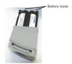
4. Replace the tray, making sure the tray snaps into place. Repeat this process for the other battery tray.
