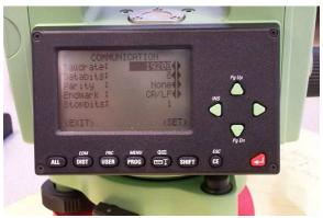
Then run SurvCE and in Equip / Total Station set it to Manufacturer: Leica TPS Series (Direct) and Model: TPS 300/400/800
