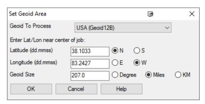
5. When prompted to name your Geoid file, please make sure to type in a unique geoid name, which relates to the location which the geoid's Lat/Long is centered on. For example, the City Name and 2012B for the Geoid model {i.e. - Boston\_MA2012B or Maysville\_2012B}.
