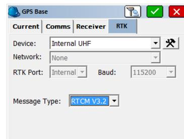
6) Tap the "wrenches" next to "Device: Internal UHF" and fill out the radio using the settings below then tap the Green Check:
