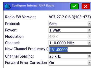
\*\*\* If you used a custom frequency for the base other than 461.0000 you will need to type in the same exact frequency you used for your Base Radio in the "New Channel Frequency" box below "1: 0MHz" to make sure your Rover radio is properly matched with the base radio
