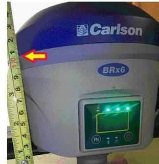
3) Then tap the Receiver tab and tap next to "Slant" and measure up to the line where the top Blue cap meets the bottom Grey housing as shown in the image to the right with the Arrow symbol to use for your Antenna height
