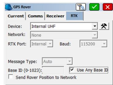
12) Tap the "wrenches" next to "Device: Internal UHF" and fill it out using the exact same settings as the ones you used for the base setup above then tap the Green Check to save your changes
