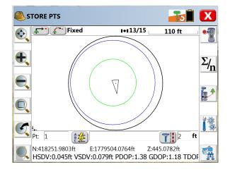
**Example 5:** Some receivers also detect instability in the compass which can lead to inaccurate compass readings. When **Check for Unit Motion** is checked in Equip/Configure/IMU tab, an orange icon will be used to indicate that instability is detected. When the read button is pressed in this state, SurvCE will wait up to 1 second for the receiver to stabilize before storing the reading.
