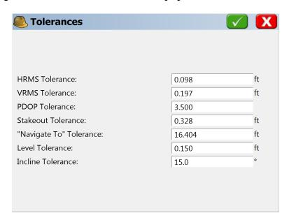
The **Level Tolerance** defines the amount of error that will be accepted when storing points. The tolerance is defined as the amount of distance error allowable on the ground, and thus is a function of both the incline of the pole and the rod height.
