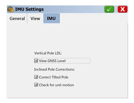
The **Incline Tolerance** in the tolerance menu defines the maximum amount of tilt allowable in this mode. Most receivers begin to lose accuracy when tilted more than 20 degrees.
