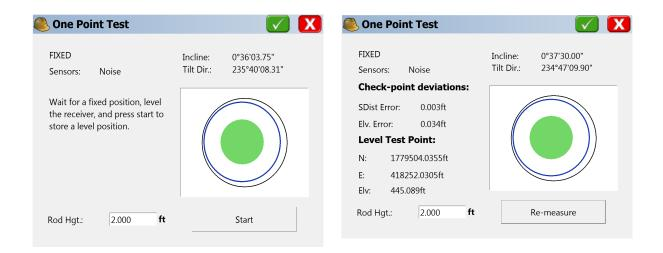
To use the feature, make sure your Rover has a FIXED solution shown in the upper left, then level the receiver and press the Start button to take a level reading.
