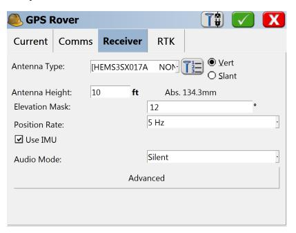
Individual IMU features of SurvCE are controlled in **Equip->Configure**, on the IMU tab:
