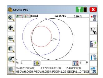
**Example 2:** The red icon in the topbar indicates that the receiver is tilted too far to correct for tilt, as configured in the tolerances dialog by the Incline Tolerance (for example, more than 20 degrees). The bubble level also shows that the receiver is very unlevel. No point can be stored.
